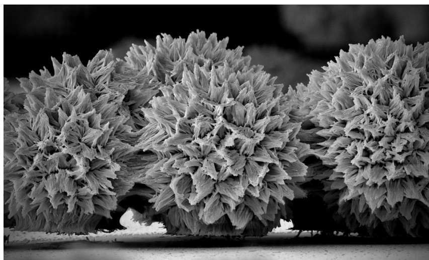
Fig. 1. SEM image of hierarchically organized supraparticles self-assembled from covellite nanosheets.
